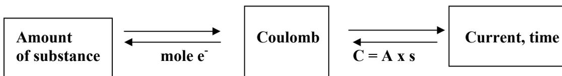
In the electrolysis of molten NaCl discussed above, the reduction of one mole of  $\text{Na}^+$  at cathode requires one mole (1 Faraday) of electrons, i.e., 96,500 C:
