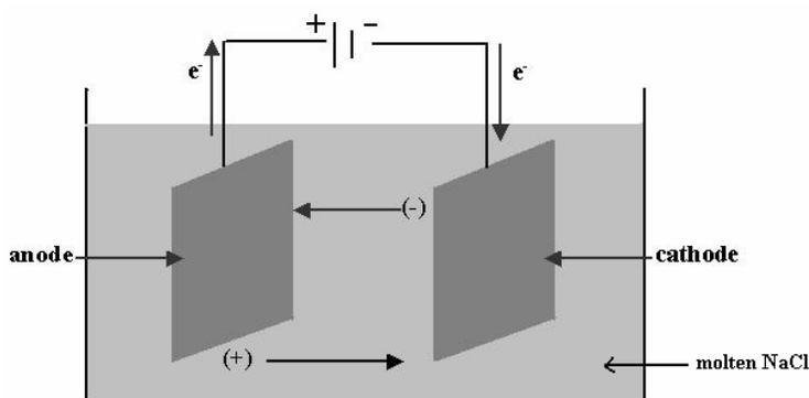
In molten sodium chloride (NaCl), there are two ions, namely, cation  $\text{Na}^+$  and anion  $\text{Cl}^-$ . At the anode, the oxidation of chloride ion takes place by depositing two electrons and forming a pure chlorine gas. At the same time, the reduction of sodium ion takes place at the cathode forming a pure sodium metal. The reactions at both electrodes are given below:
